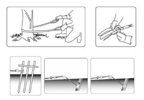
Step 5: Couple hook to anchor point. If unable to find anchor point, make one using accessory.
