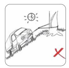
**9.** Do not leave loads unattended,wire rope could come loose from the drum, as the wire rope attachment to the drum is not designed to hold a load.
