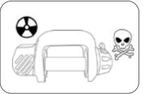
If used near chemicals, corrosive gas or explosives may cause an explosion. Exposure to salt or acids may cause malfunctioning.
