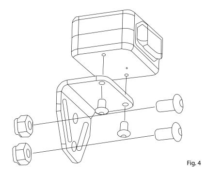
**1.** Switch is usually installed on left handlebar on ATVs. If installing on UTV or SxS, use supplied bracket and hardware as shown in Fig. 4. This bracket can be placed in any location that is convenient.
