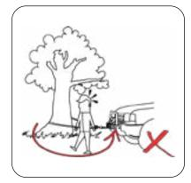
**5.** During winching operation always be aware of stability of vehicle and load during winching, keep others away. Alert all by standers of an unstable condition.
