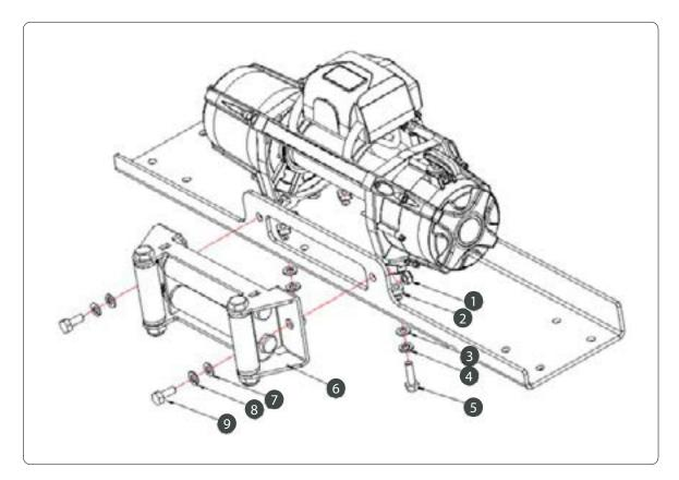
**1.** 1) Install suitable mounting bumper or mounting plate in required position. Winch must be mounted with direction of pull perpendicular to mounting bolt fixings. Steel plate should be at least 6mm thick.
