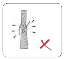
**3.** Always inspect winch rope, hook, and slings before operating winch. Frayed, kinked or damaged winch rope must be replaced\ immediately.
