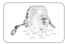
Exposure to sand may cause malfunctioning.
