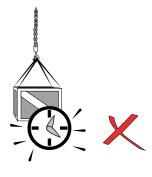
9. Do not leave the load lifted for long periods of time. It may cause deformation of the equipment and increase the risk of an accident.
