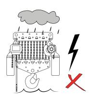
6. Do not use the hoist if exposed to rain, snow or lightning.
