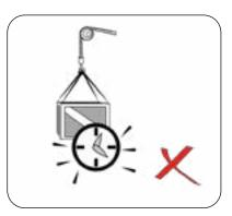
**9.** A heavy object must not stay up in the air for an extended period of time, it may cause girder deformation and/or cause an accident.
