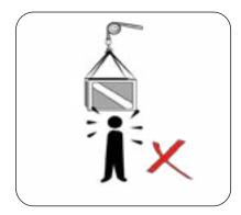
**1.** Do not exceed rated load. Make sure you know and the ability to lift maximum capacity of your equipment.
