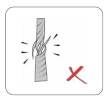
**3.** Check frequently the hoist's steel chain. In case of any damage, replace it.
