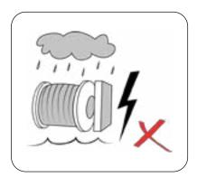
**6.** Do not use the hoist under the rain. Do not wet the engine or the switch.
