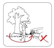
**5.** During winching operation always be aware of stability of vehicle and load during winching, keep others away. Alert all bystanders of an unstable condition.
