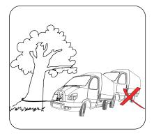
**1.** Do not exceed winch or winch rope rated capacity.
