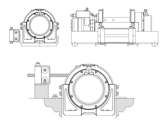
The diagrams show the mounting dimensions for the 8000 - 18000LB. The side and feet mounting hole positions are designed to allow the winch to be interchangeable with the most popular 8000 - 18000LB units currently available. The diagram below shows the 8000-18000LB mounted on a flatbe mounting kit, shown with roller fairlead. If a mounting plate is not used, the surface must be flat within 0.5mm and sufficient stiff to prevent fixing. A minimum of 6.0mm tick steel plate should be used.
