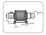
Exposure to sand may cause malfunctioning.
